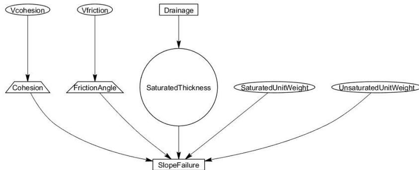
Figure 7: The CN model of an infinite slope.
