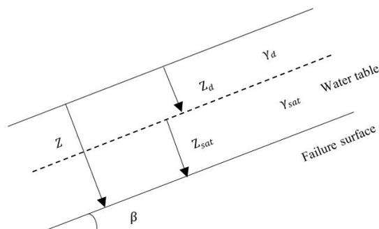
Figure 5: An infinite slope.
