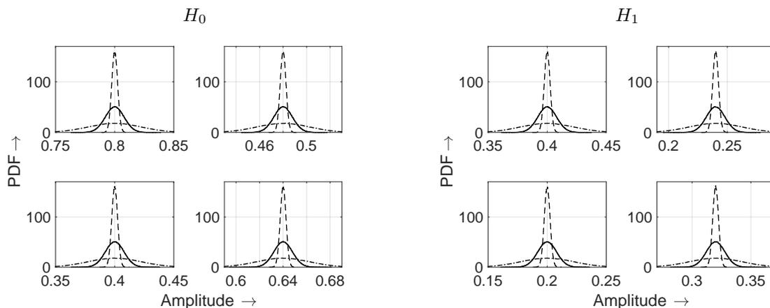
Figure 2: Empirical probability density functions of the estimated MIMO channel taps comparing different pilot sequence lengths — dash-dotted line:  $L_s = 5$ , solid line:  $L_s = 33$ , dashed line:  $L_s = 321$
