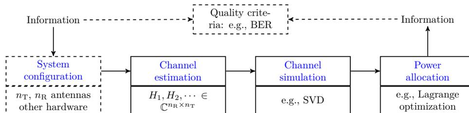
Figure 1: Subprocesses during the modeling and simulation of a (MIMO) digital channel
