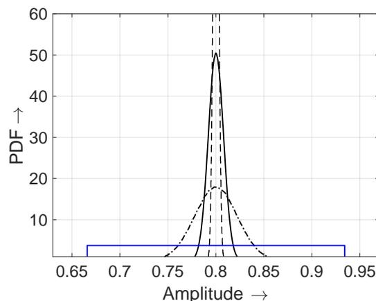
Figure 3: Channel coefficient  $H_0(1,1)$ : Empirical PDFs for pilot sequence lengths  $L_s = 5$  (dash-dotted line),  $L_s = 33$  (solid),  $L_s = 321$  (dashed) and the interval enclosure (blue line) for  $\pm 3\sigma$
