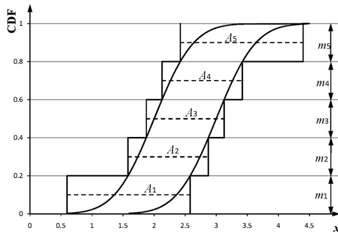
Figure 2: A P-Box defined by bounding lognormal distribution with mean of [2.47, 11.08] and standard deviation of [2.76, 12.38] (**Enclosure Discretization**)
