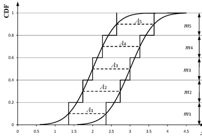
Figure 3: A P-Box defined by bounding lognormal distribution with mean of [2.47, 11.08] and standard deviation of [2.76, 12.38] (Mid-point Discretization)
