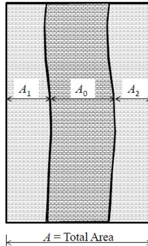
Figure 3: An example of spatial distribution of damage areas on a façade (the darker area represents a higher probability for damaged blocks)
