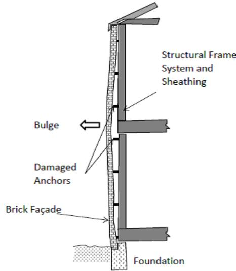
Figure 2: Damaged metal anchor causing brick wall to bulge out
