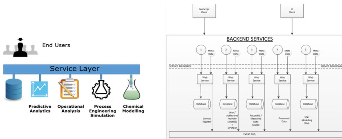
Figure 2: Schematic of the service oriented architecture of the digital twin framework. Showing the high level components (left) and the service Oriented Architecture (right). The R service is integrated as a client and the process model is integrated as a web service (NNL Modelling Web) as part of the High Level Architecture. A more detailed description of the architecture is presented in section 3.3 and 3.4.
