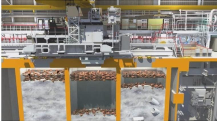
Figure 1: 3D Render of the Magnox Swarf Storage Silos (Source: Sellafield Ltd, original video on ITV.com). The OR model described in 3.4.4 uses 3D visualisation to demonstrate potential bottlenecks in decommissioning activities. The image shows three of the silos which contain a mix of solid debris, settled solids and liquid wastes. The digital twin has been designed to support operations for the removal and treatment of the liquid waste.
