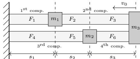
Figure 3: Front structure of a vehicle with four components, three masses, two load paths, and three sections, compare [2]
