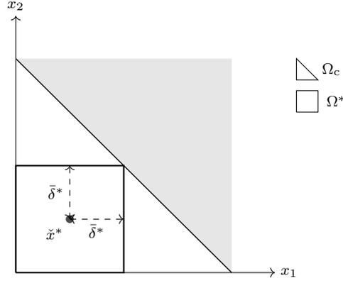
Figure 2: Solution space  $\Omega^*$  defined by the robust design  $\check{\mathbf{x}}^*$  and the maximal tolerance  $\bar{\delta}^*$
